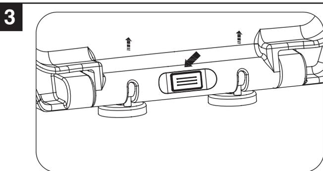
3. Open the seat and cover. Push the center push button to release seat and cover. Pull upwards the seat and cover to take it off the hinges.
