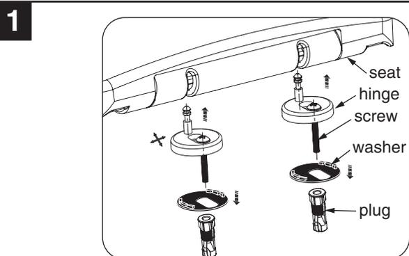
1. Insert the plugs into the fixing holes of the toilet. Install rubber washer on bottom of hinge. Click the hinges into the seat & cover fixing holes.
