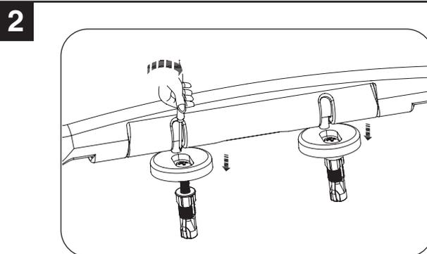
2. Close the seat and cover onto the toilet and adjust seat and cover to a proper position. Tighten the screws firmly with a screwdriver.
